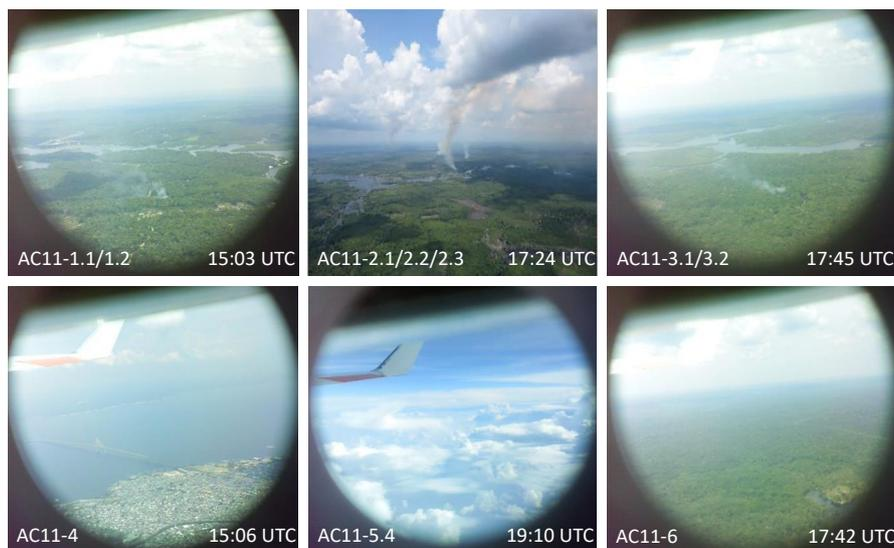
**Figure 7.** Images taken by the mini-DOAS camera during events 1–6 (as indicated in fig. 6 and 8) for the flight AC11 with the UTC time given in each image. The second image was taken from the respective flight report. The video camera points into the same direction as the three limb telescopes of the mini-DOAS spectrometer, however with a much larger field of view of  $\sim 46^\circ$  width.
