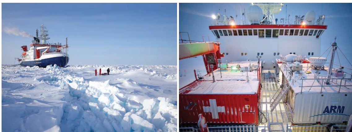
Figure 2. Polarstern drifting in the Arctic ice on 10 April 2020 (left panel) and measurement containers for in situ aerosol monitoring (the two first containers on the left side and the first container on the right side), and for remote sensing of aerosols and clouds (right panel). The OCEANET container of TROPOS is the third one on the left side. The ARM mobile facility (AMT-1) is shown on the right side. The photographs are taken by Michael Gutsche (CC-BY 4.0), AWI.
