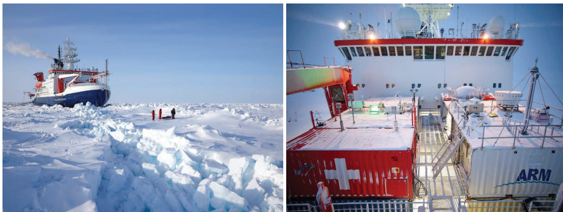
Figure 2. Polarstern drifting in the Arctic ice on 10 April 2020 (left panel) and measurement containers for in situ aerosol monitoring (the two first containers on the left side and the first container on the right side), and for remote sensing of aerosols and clouds (right panel). The OCEANET container of TROPOS is the third one to the back on the left side (with the bright spot on the roof caused by green laser light). The ARM mobile facility (AMT-1) is shown on the right side. The photographs are taken by Michael Gutsche (CC-BY 4.0), AWI.
