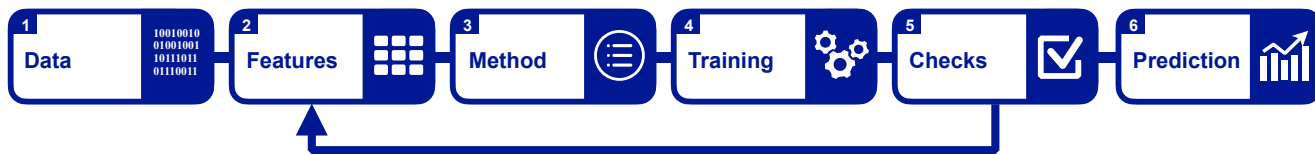
Figure 1. Schematic of our machine learning workflow: The raw input data is converted into molecular representations (referred to as features in this figure). We then set up and train a machine learning method. After evaluating its performance in step 5, we may adjust the features. Once the machine learning model is calibrated and trained, we make predictions on new data.
