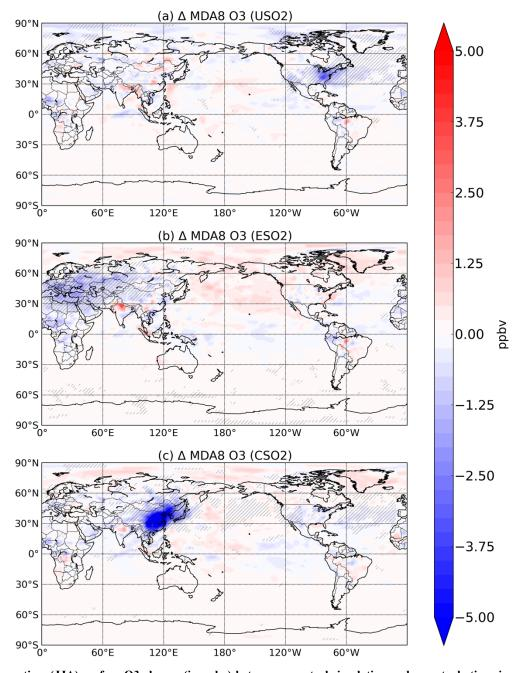
Figure 5: Summertime (JJA) surface O3 change (in ppbv) between a control simulation and a perturbation simulation in which anthropogenic SO2 emissions are removed over a certain region: (a) US, (b) Europe, and (c) China. Hatching denotes statistical significance according to a Student's t-test at the 95% confidence level.
