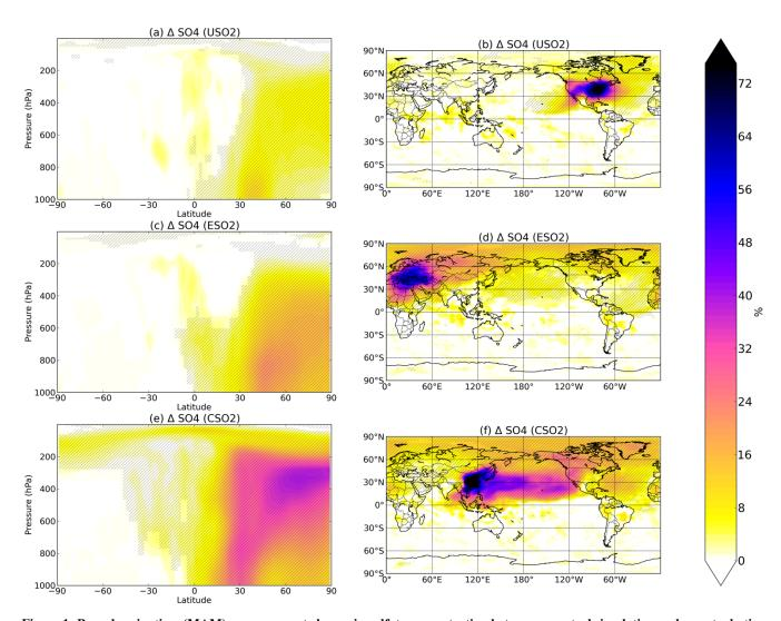
Figure 1: Boreal springtime (MAM) mean percent change in sulfate concentration between a control simulation and a perturbation simulation in which anthropogenic SO2 emissions are removed over a certain region: (a,b) US, (c,d) Europe, and (e,f) China. Hatching denotes statistical significance according to a Student's t-test at the 95% confidence level.
