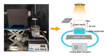
Photochemistry reaction device. The inside diameter of the reactor is approximately 11 cm, and the height is approximately 18 cm. The reactor is connected to a cooling-water circulator to ensure that the water temperature in the reactor was constant and the water temperature is set to 8 °C (Chen et al. 2021).
