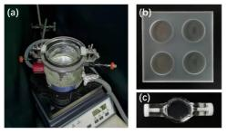
**Figure S2.** Schematic diagrams of the photochemical devices. (a) The reactor is used for maintaining the reaction environment. (b) The capsule is used for the experiment of triplet state inducing singlet oxygen. The size of quartz plate is  $35 \times 35$  mm<sup>2</sup>. The size of the tanks is a radius of 5.6 mm and a depth of 2.5 mm. (c) The capsule is used for triplet state experiments. The reactor is made of quartz. The plugs are made of Teflon. The internal volume is 200 µL.
