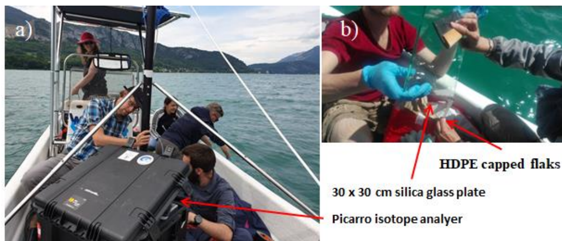
335 Figure 6. Illustration of the shipboard payload with operators. a) The CRDS isotope analyser is on board the boat. b) The surface microlayer of the lake is sampled using both a silica glass plate and a high-density polyethylene (HDPE) capped flask.
