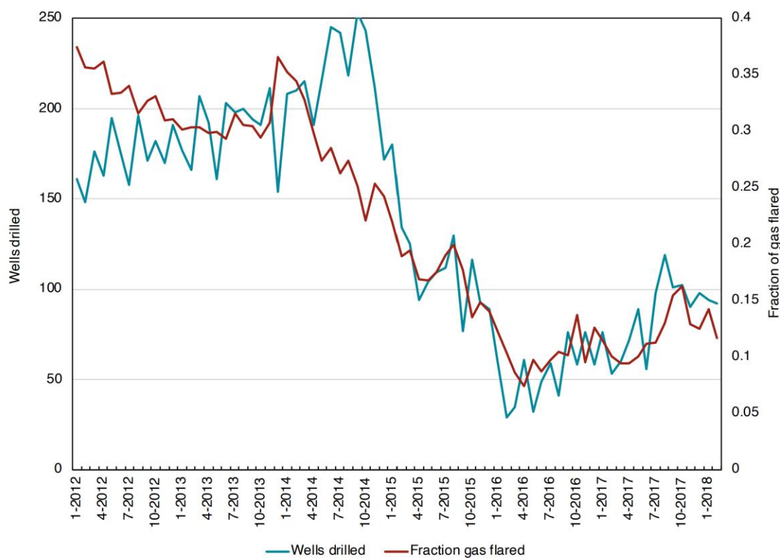
690 Figure F1. Number of wells drilled versus fraction of total gas production flared in the Bakken region (North Dakota, U.S.A.) from 2012 - 2017. Similar to trends observed in the Permian, there was a strong correlation between wells drilled and fraction of gas flared with both values decreasing rapidly when oil prices crashed in 2014.
