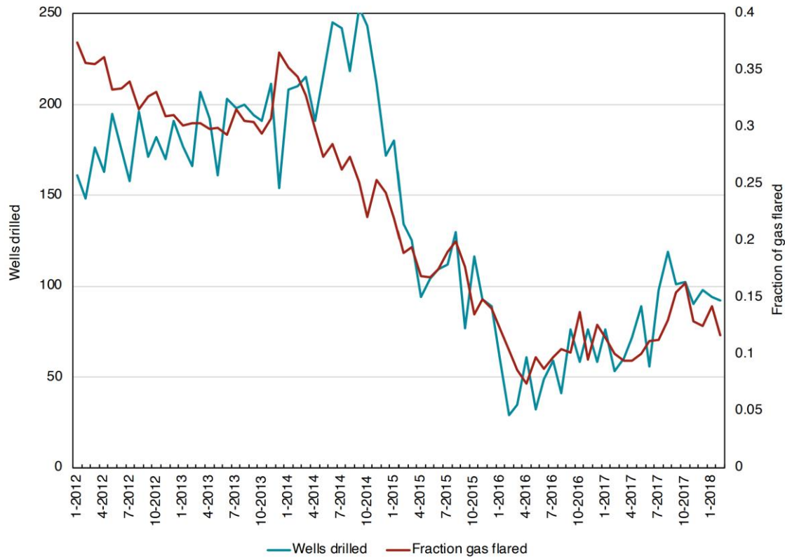
645 Figure F1. Number of wells drilled versus fraction of total gas production flared in the Bakken region (North Dakota, U.S.A.) from 2012 - 2017. Similar to trends observed in the Permian, there was a strong correlation between wells drilled and fraction of gas flared with both values decreasing rapidly when oil prices crashed in 2014.
