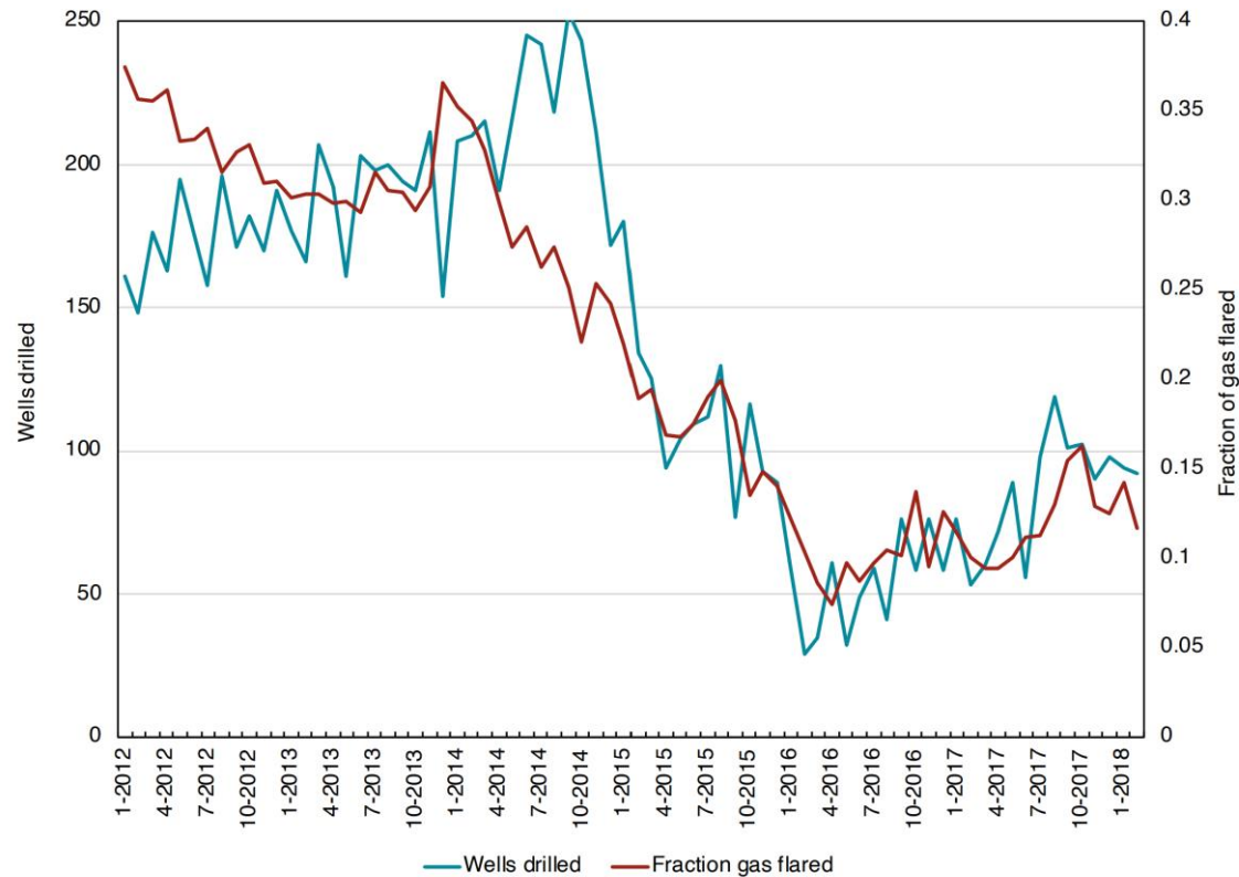
695 Figure F1. Number of wells drilled versus fraction of total gas production flared in the Bakken region (North Dakota, U.S.A.) from 2012 - 2017. Similar to trends observed in the Permian, there was a strong correlation between wells drilled and fraction of gas flared with both values decreasing rapidly when oil prices crashed in 2014.
