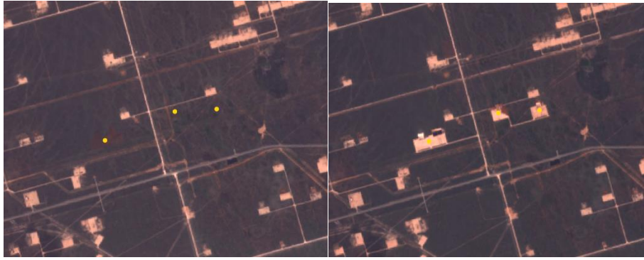
Figure C4. Example of an area where new development was found, before (top) and after (bottom) shown in Sentinel-2 785 imagery (ESA, 2020). Points in yellow indicate the locations of new well pad development.
