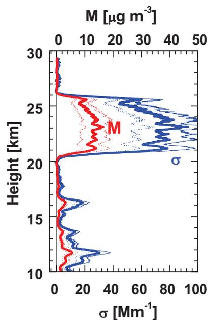
**Figure 10.** Smoke observation with lidar in the stratosphere over Punta Arenas on 29 January 2020 (see Fig. 1) in terms of particle extinction coefficient  $\sigma$  and particle mass concentration  $M$ . Extinction coefficients were obtained by multiplying the respective backscatter coefficients with a lidar ratio of 95 sr. Typical uncertainties of 25% and 35% in the extinction and mass retrievals, respectively, are shown as thin dotted lines.
