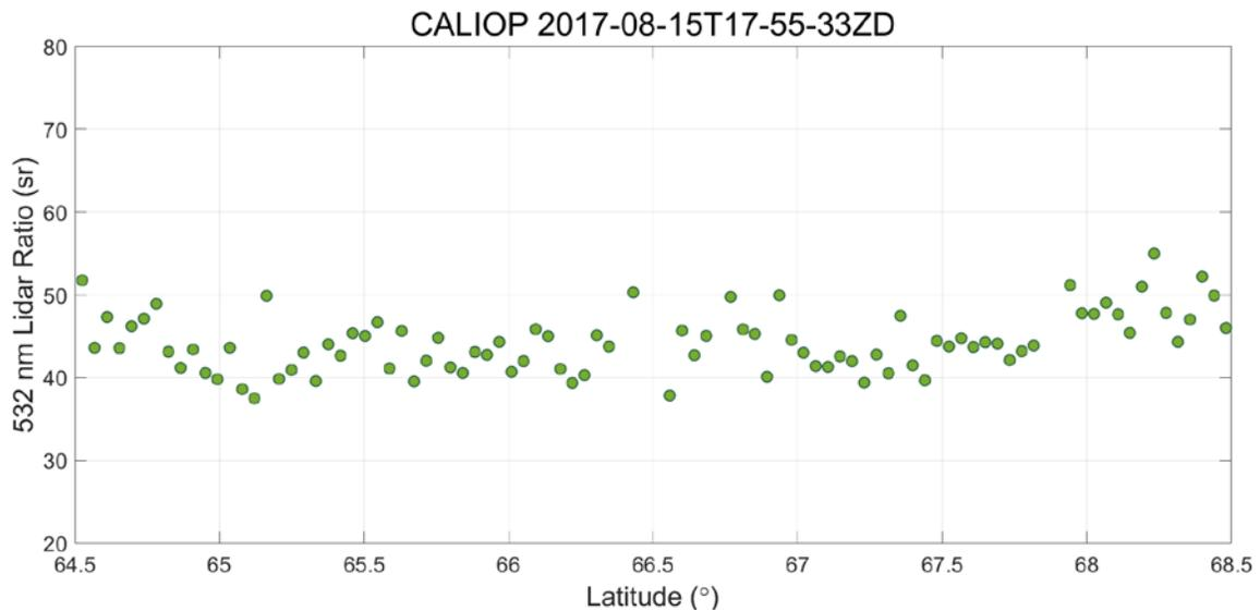
Figure 3: optimized values of effective lidar ratio,  $\eta S = 1 / 2\gamma'$  for the opaque portions of the smoke layer shown in Figure 2.
