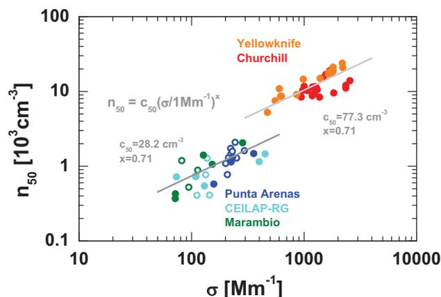
**Figure 9.** Relationship between smoke extinction coefficient  $\sigma$  (532 nm) and particle number concentration  $n_{50}$  for the different AERONET data sets (fresh smoke vs aged smoke). Clear differences for fresh and aged smoke are visible. More details in the text.
