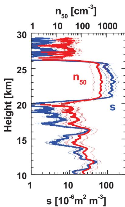
**Figure 11.** Retrieval results for 29 January 2020 in terms of surface area  $s$  and particle number concentration  $n_{50}$  (proxy for CCN) with error margins representing typical uncertainties (30% for  $s$  and a factor of 2 for  $n_{50}$ ).
