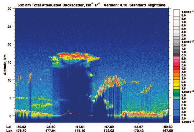
**Figure 13.** CALIPSO lidar observations of a stratospheric smoke layer between 13.5–17.5 km height over New Zealand (35–42°S) on 1 January 2020 around 13:00 UTC (CALIPSO, 2020a). The plume was injected during a strong and long-lasting pyro-Cb event on 30–31 December 2019 (Ohneiser et al., 2020) and then ascended by several kilometers within the next 24–36 hours.
