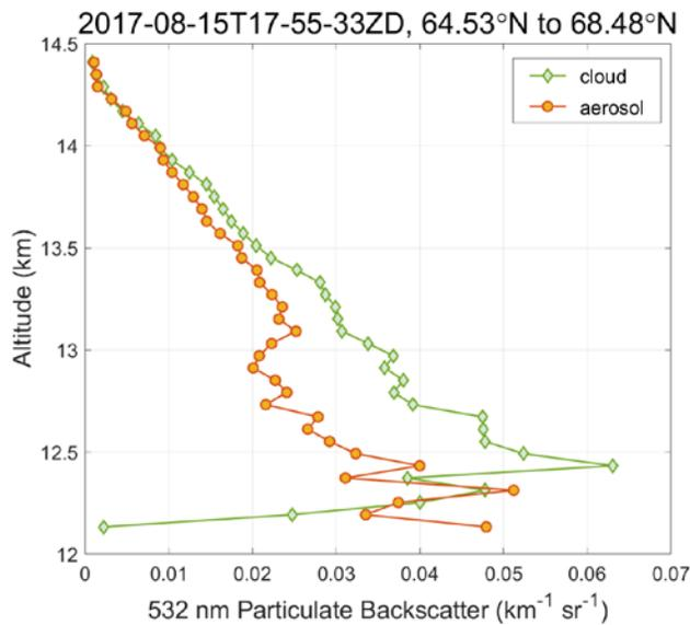
Figure 4: backscatter coefficients retrieved within the smoke layer shown in Figure 2.
