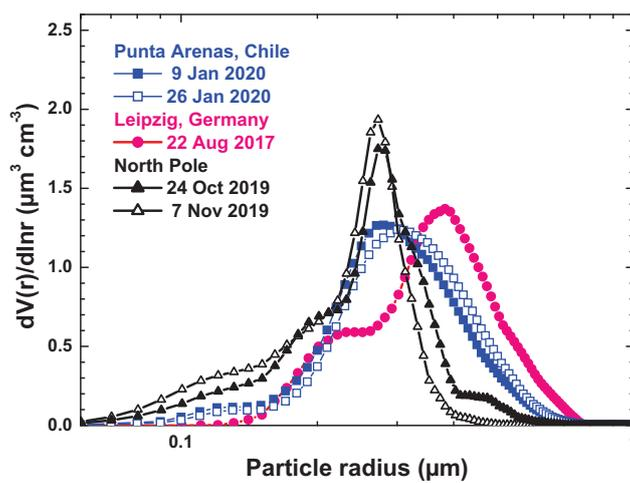
**Figure 5.** Lidar-derived normalized volume size distributions of stratospheric smoke particles found for Canadian smoke over Leipzig, Australian smoke over Punta Arenas, and Siberian and Alaskan smoke over the North Pole region.
