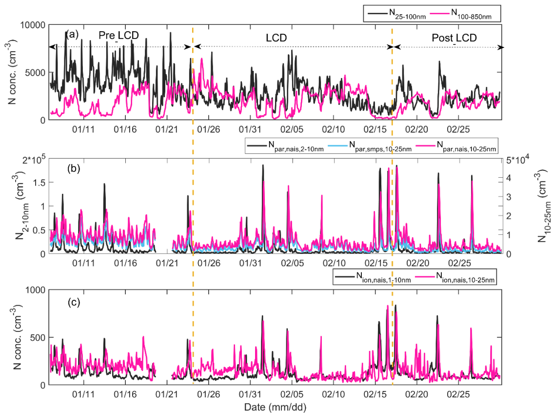
Fig. 3. Time series of hourly mean of the number concentrations for different size ranges, including 25–100 nm and 100–850 nm, from SMPS data (a); 2–10 nm particles from NAIS and 10–25 nm particles from both NAIS and SMPS
