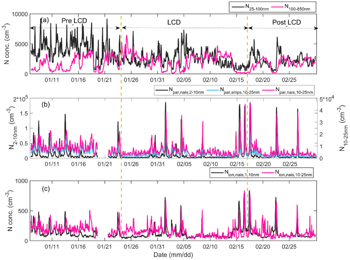
Fig. 3. Time series of hourly mean of the number concentrations for different size ranges, including 25–100 nm and 100–850 nm, from SMPS data (a); 2–10 nm particles from NAIS and 10–25 nm particles from both NAIS and SMPS (b); 1–10 nm and 10–25 nm positive ions from NAIS (c).
