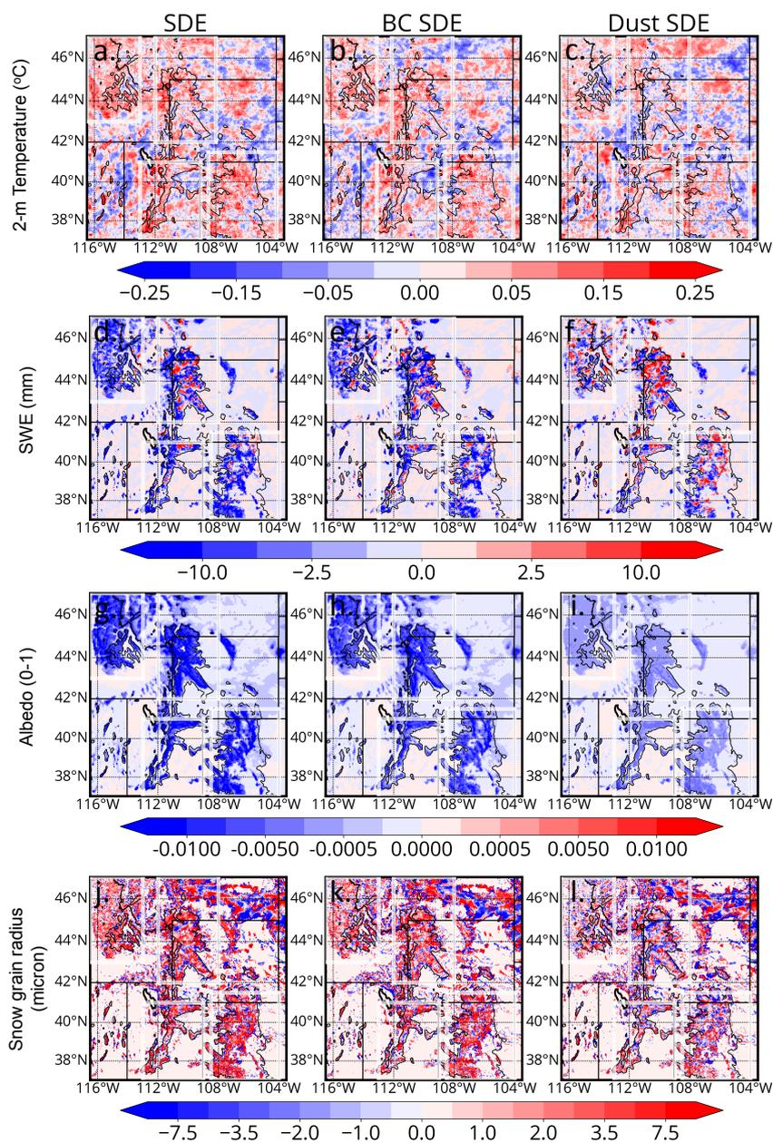
1010 **Figure 8.** March through June averaged SDE-induced anomalies in (top row) 2-m temperature, (second row) SWE, (third row) albedo, and (bottom) snow grain effective radius in the top snow level for (first column) BC+dust, (second column) BC, and (third column) dust. The thin black contours denote the 2,200 m elevation contour.
