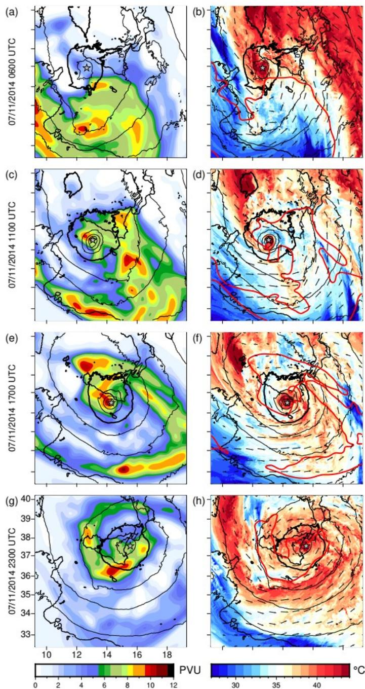
**Figure 5:** Potential vorticity at 300 hPa (colour scale) and SLP (isocontours every 4 hPa, the 1000 hPa isobar is in bold), (a, c, e, g) and equivalent potential temperature ( $^{\circ}\text{C}$ , colour scale) and wind at 850 hPa, SLP, and 6 PVU at 300 hPa isocontours (red), (b, d, f, h) from the NOCPL simulation.
