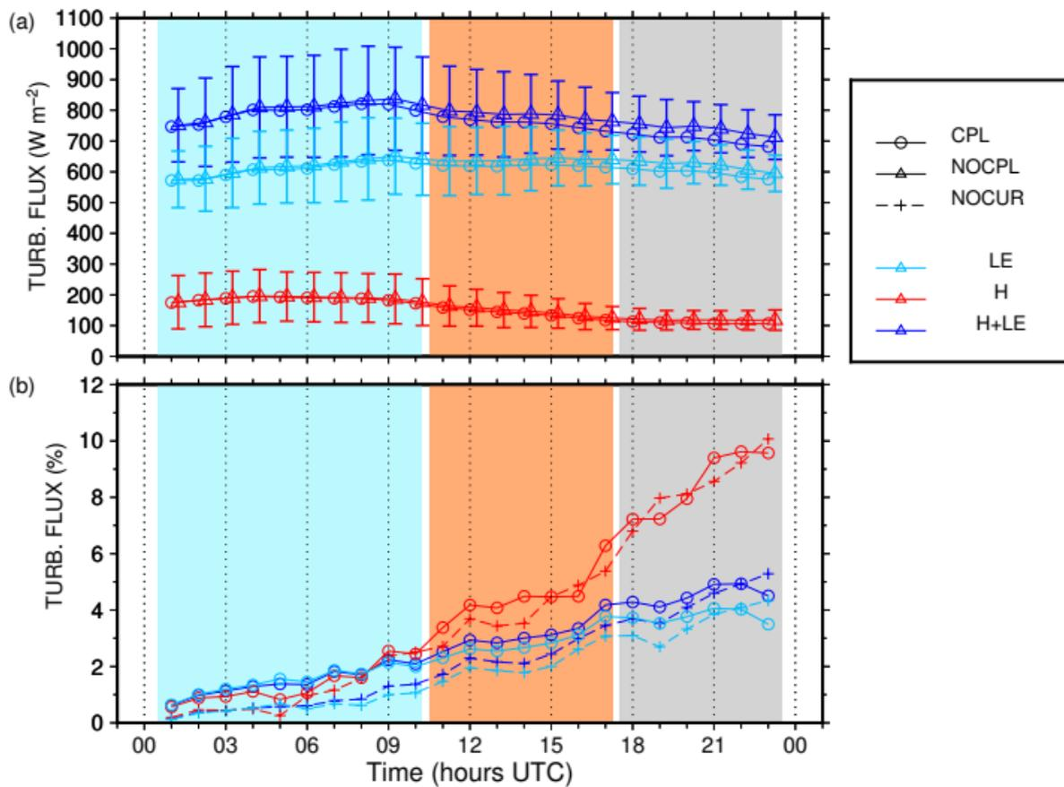
**Figure 9:** Time series of the mean values and standard deviation (error bars) of the total turbulent heat flux (blue), latent (cyan) and sensible heat flux (red) in the CPL (open circles) and NOCPL (triangles) simulations (a) and of the mean difference between CPL and NOCPL turbulent fluxes (open circles, same colour code) and between NOCUR and NOCPL turbulent fluxes, in percent relative to the NOCPL values (b) on the EF600 area.
