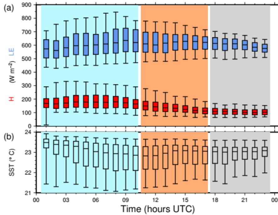
**Figure 10:** Time series of the median values of latent (blue) and sensible heat fluxes (red, a) and of SST (b) on the EF600 area (see text),
