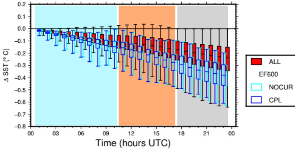
880 **Figure 8:** Time series of the median differences between the SST in the CPL and NOCPL simulations, on the whole domain (red) and on the EF600 area (blue, see text for definition), on the 7 November. The boxes indicates the 25 and 75% quantiles and the whiskers the 5 and 95% quantiles. The SST differences on the EF600 area between the NOCUR and NOCPL simulations are also shown (cyan). Some of the boxes have been slightly shifted horizontally for clarity.
