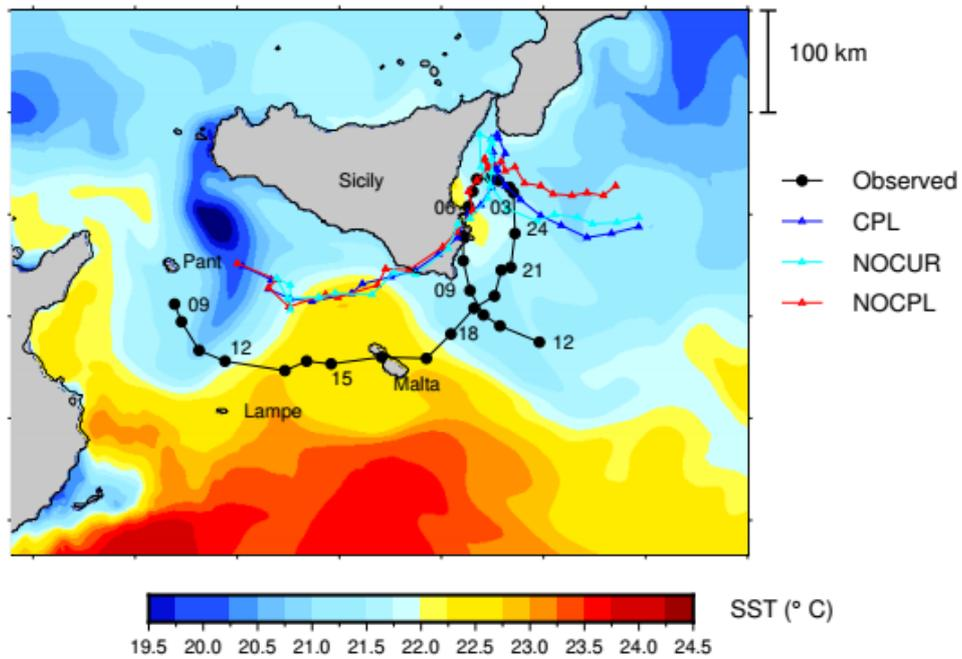
765 **Figure 3:** Comparison of the simulated tracks (triangles) of the non-coupled run (NOCPL, red), coupled run with SST only (NOCUR, cyan) and fully coupled run (CPL, blue) with the best track (black closed circles) based on observations as in Cioni et al., (2018). The position is shown every hour with time labels every 3 h, starting at 09:00 UTC on 7 November until 12:00 UTC on 8 November. In colours, initial Sea Surface Temperature (SST, °C) at 01:00 UTC on 7 November.
