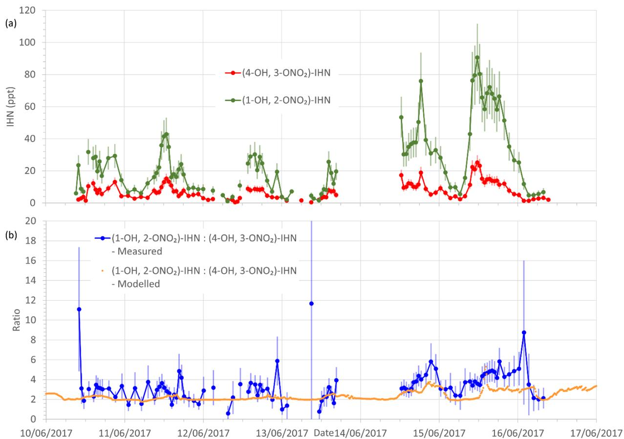
685 **Figure 3.** (a) Measured  $\beta$ -IHN mixing ratios. (b) Measured and modelled ratio (1-OH, 2-ONO<sub>2</sub>)-IHN:(4-OH, 3-ONO<sub>2</sub>)-IHN. Error bars are the measurement uncertainties (see Sect. 3.3 for details).
