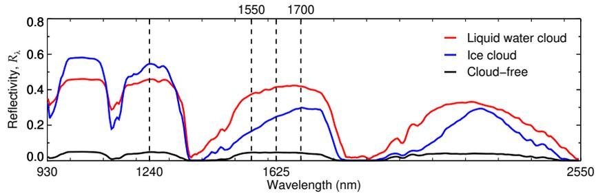
**Figure 1.** Reflectivity spectra of a pure liquid water cloud and a pure ice cloud of optical thickness 12 compared with a clear sky spectrum in the wavelength range measured by AISA Hawk. The vertical dashed lines indicate the wavelengths needed to calculate the slope phase index (1550 - 1700 nm), and to retrieve the cloud optical thickness (1240 nm) and effective radius (1625 nm)
