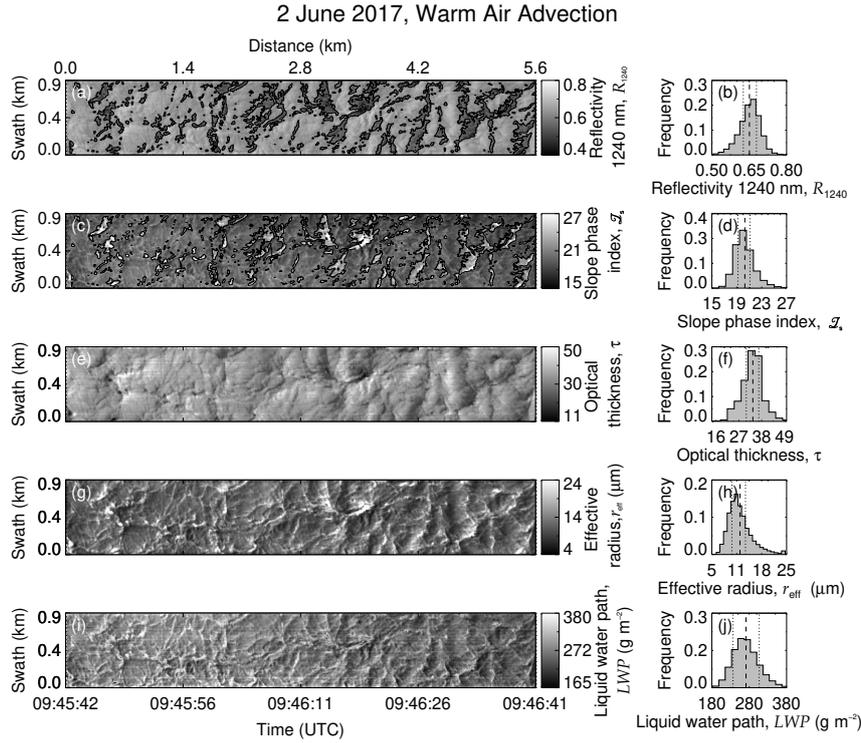
**Figure 6.** AISA Hawk measurement on 2 June 2017. Cloud top reflectivity (a), slope phase index (c), retrieved optical thickness (e), retrieved effective radius (g) and liquid water path (i). The overlaid contours in (a) and (c) separate the cloud central regions from the cloud edges. The frequency of occurrence histograms are displayed on the corresponding right-hand figures (b, d, f, h, j). The dashed line indicates the mean value and the dotted lines show its 25th and 75th percentile.
