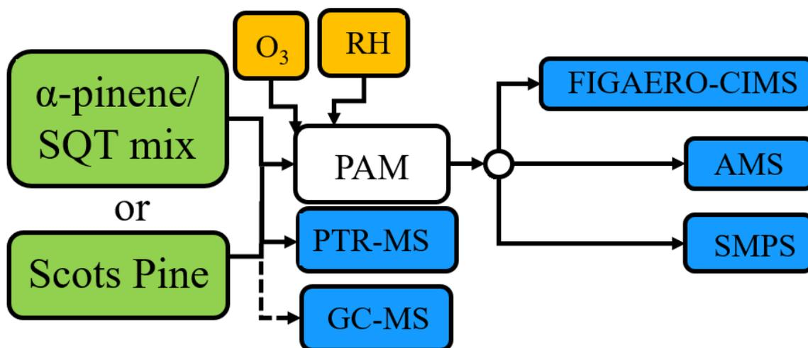
Figure 1: Measurement setup used in the experiments. Abbreviations in the picture are explained in the main text (Sect. 2), except for ozone-containing air (O<sub>3</sub>) and humidified air (RH).
