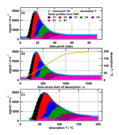
**Figure 2:** Measured total ion thermogram colour coded with the contribution of PMF model output factors for the mediumOC,  $t_{evap} = 4$  h, wet case plotted vs data point index (a), time since start of desorption (b), and desorption temperature (c). Note that the desorption temperature ramp (b) is not increasing linearly after ~1000 s. This "soak" period ensures that all organic material is removed from the filter before the next collection.
