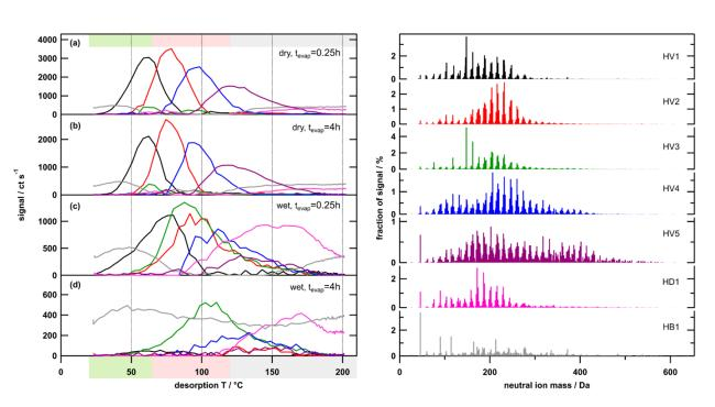
**Figure 7:** Temperature profiles (left) and factor mass spectra (right) for the 7-factor solution for highOC case. Each factor mass spectrum is normalised. The colour code is the same for both panels Background colour in the left panel indicates volatility classification derived from  $T_{max}$  - C\* calibrations (green: SVOC, red: LVOC, grey: ELVOC).
