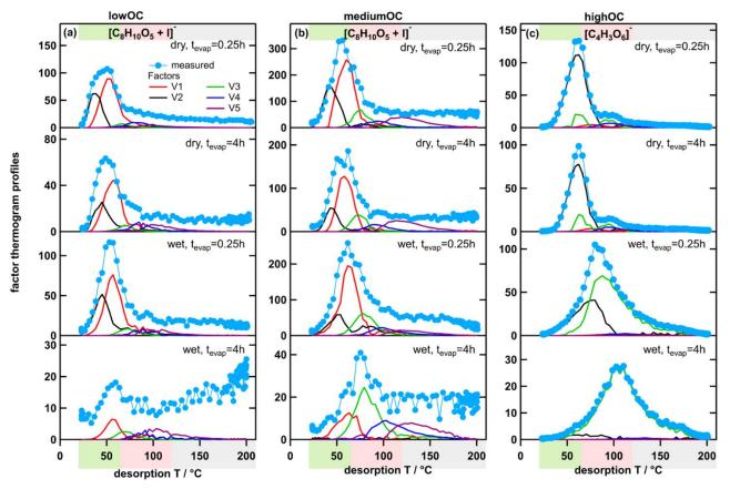
**Figure 9:** Measured ion thermograms and factor thermogram profiles for ion  $[C_8H_{10}O_5+I]^-$  in the low- (a) and mediumOC cases (b) and  $C_4H_3O_6^-$  in the highOC case (c). Note that to reduce clutter in the graph only V-type factors are displayed. Thus, coloured lines will not add up to the measured values (light blue) if the sample to background ratio was low (e.g. bottom panel in a).
