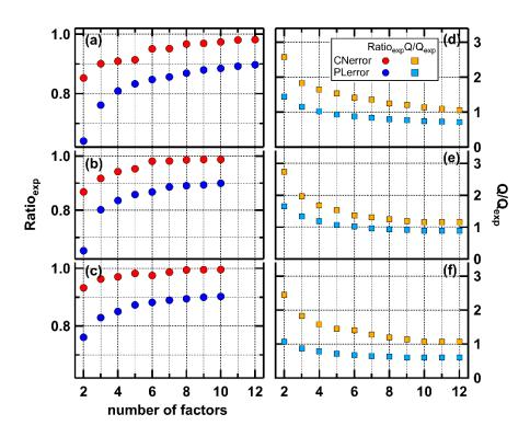
**Figure 3:** Fraction of explained variance (*Ratio*<sub>exp</sub>, left) and  $Q/Q_{exp}$  values (right) for the low- (a), medium- (b) and highOC- dataset for PLerror (blue) and CNerror(red).
