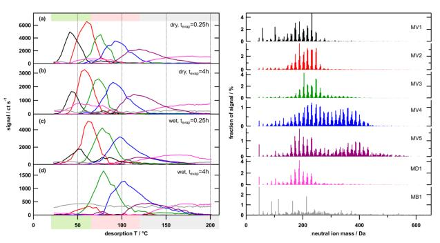
**Figure 6:** Temperature profiles (left) and factor mass spectra (right) for the 7-factor solution for the mediumOC case. Each factor mass spectrum is normalised. The colour code is the same for both panels. Background colour in the left panel indicates volatility classification derived from  $T_{max}$ -C\* calibrations (green: SVOC, red: LVOC, grey: ELVOC).
