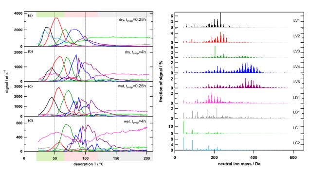
**Figure 5:** Temperature profiles (left) and factor mass spectra (right) for the 9-factor solution for the lowOC case. Each factor mass spectrum is normalised. The colour code is the same for both panels. Background colours in the left panel indicate volatility classifications according to Donahue et al. (2006) derived from  $T_{max}$ -C\* calibrations (green: SVOC, red: LVOC, grey: ELVOC).
