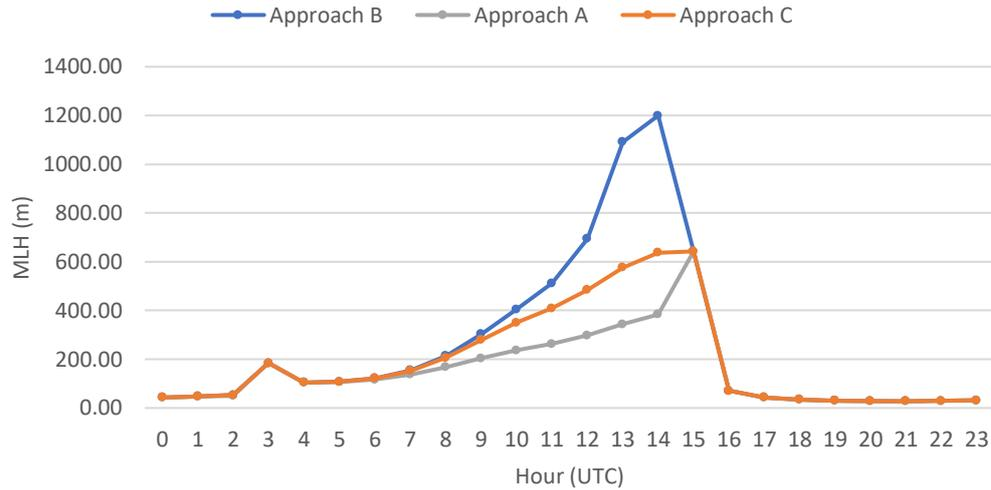
**Figure 2: An example of the effective MLH evolution for different approximation of  $R_n$  concentration in the residual layer. Approach C was used in the model. Spring average diurnal profile of  $C_{R_n}$  in Ljubljana was used for comparison.  $E_{R_n}$  was fixed and does not match the values finally used in the manuscript.**
