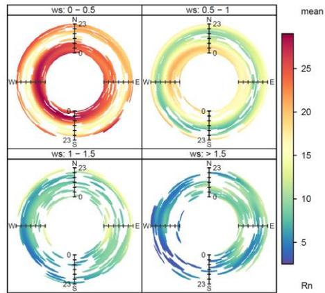
**Figure 1: Vipava valley location: a) Digital elevation model of the Vipava valley with marked measurement sites, b) monthly wind rose, c) monthly wind rose for a subset of wind speed below 2 m/s, d) polar annulus plot shows how Rn concentration (color code in  $Bq/m^3$ ) vary by wind direction and hour of day .**
