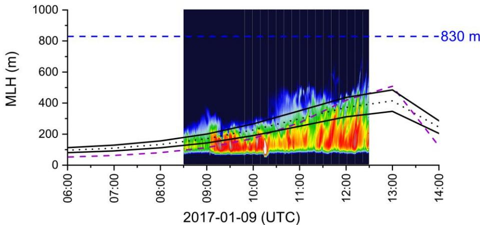
**Figure 3: Comparison of effective MLH calculated using the Approach A (black dotted line), B (violet dashed line) and C (black solid line, min and max). Due to low  $R_n$  concentration in the residual layer from the previous day, the Approach A and C gives similar results in this case.**
