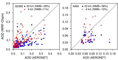
**Figure 7.** Hourly AOD from the measurements of AERONET and simulations by WRF-Chem at the two sites over the TP (QOMS, 86.56°E, 28.21°N; NAM, 90.96°E, 30.77°N) for April, 2016.
