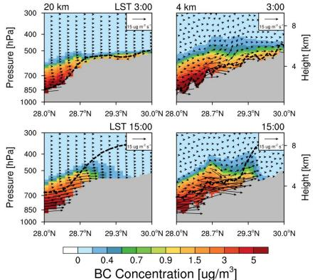
**Figure 11.** Latitude-height cross section of BC flux (vector) along the valley (shown as the black line in Fig. 3) from the simulations at 20 km and 4 km resolutions at local time (LT) 03:00 and 15:00 averaged for April 5-20, 2016. Contour represents the BC concentration.
