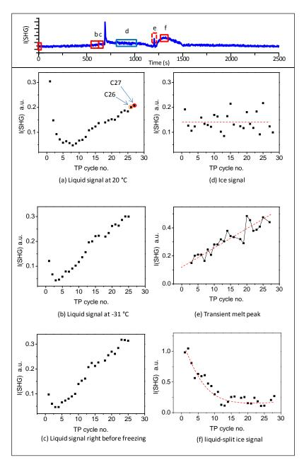
Figure 4: Upper panel: a sample plot of SHG vs. time during the standard TP. Lower panel: The averaged SHG signal as a function of TP cycle number at the different time slots marked with red and blue rectangles in the upper panel. The red rectangle corresponds to liquid phase while the blue rectangle corresponds to ice phase. The dashed red lines on the plots are guiding lines through the data points.
