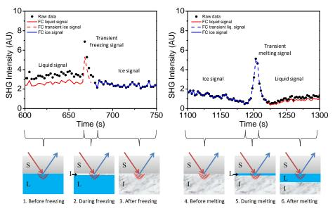
Figure 7: Upper panel: A comparison between SHG signal, corrected (continuous and dashed lines) and non-corrected (black solid circles) to the Fresnel factors, around the transient freezing peak (left panel) and around the transient melting peak (right panel) for TP cycle
