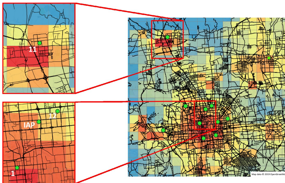
Figure 9: Spatial distribution of November and December mean MEIC Opt \text{NO}_2 emissions (all emission sectors) overlaid with Beijing road network (source: OpenStreetMap). Enlarged regions cover urban sites 1, 12 and IAP as well as suburban site 11. Right panel: © OpenStreetMap contributors 2019. Distributed under a Creative Commons BY-SA License.
