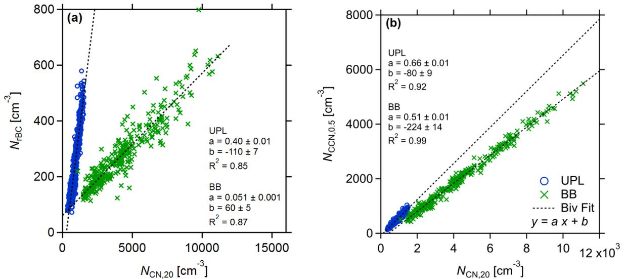
**Figure 5.** Correlation between (a) rBC particle number concentrations ( $N_{rBC}$ ) and total aerosol ( $N_{CN,20}$ ); and between (b) CCN at  $S = 0.5\%$  ( $N_{CCN,0.5}$ ) and total aerosol ( $N_{CN,20}$ ) in the UPL (blue) and in the fresh biomass burning plume (green). The dashed lines are bivariate linear regressions applied to the data sets.
