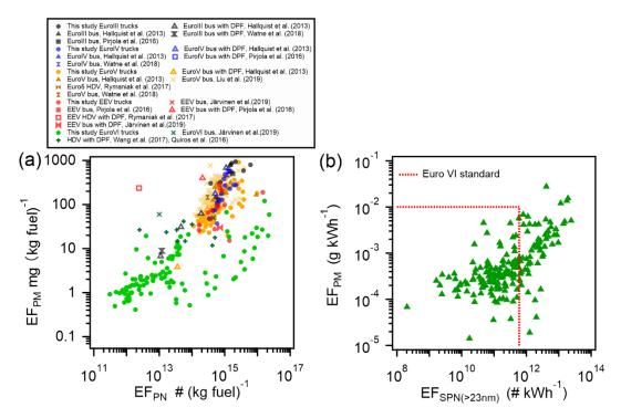
**Figure 3.** (a)  $EF_{PM}$  and  $EF_{PN}$  of individual HDTs in this study and previous studies and (b) the relationship between  $EF_{PM}$  and EF<sub>SPN</sub> of Euro VI HDTs. Red dashed lines represent Euro emission standards (horizontal: PM emission standard; vertical: SPN emission standard). Note that the comparison with the emission standard is only indicative as they are based on test cycle performance.
