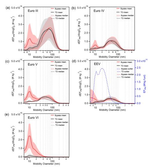
Figure 4. Mean and median size-resolved  $EF_{PN}$  and  $EF_{non-volatile PN}$  of different Euro class HDTs. Shaded regions in (a-e) represent the statistical 95% confidence interval. One HDT with extremely different EF in (d) was excluded and shown in blue.
