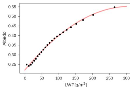
**Fig. 9** UM GA7.1 daily-mean albedo as a function of LWP over ocean between 30-60°N and outside of cyclones in equal quantiles
