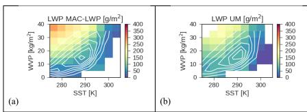
Fig. 2 MAC-LWP observed (a) and UM-simulated (b) LWP in the space of SST and WVP in the region 30°-60°N. White lines show the distribution of data in SST-WVP space.
