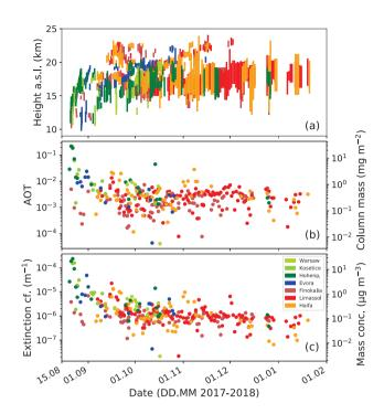
**Figure 4.** (a) Overview of all Polly observations of the stratospheric smoke layer (from base to top as colored vertical lines). For each station, one nighttime observation per day is considered. (b) Corresponding smoke layer AOT at 532 nm and estimated column-integrated smoke particle mass concentration, and (c) vertically averaged smoke particle extinction coefficient and corresponding mean particle mass concentration.
