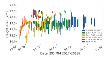
**Figure 7.** All individual day-by-day smoke observations of the 532 nm particle linear depolarization ratio (from all contributing stations, including several Lindenberg observations at 355 nm). Colors indicate different depolarization value ranges. The depolarization ratio decreased with time because of the removal of the larger non-spherical smoke particles and/or the change in the shape characteristics (from non-spherical to spherical particle shape).
