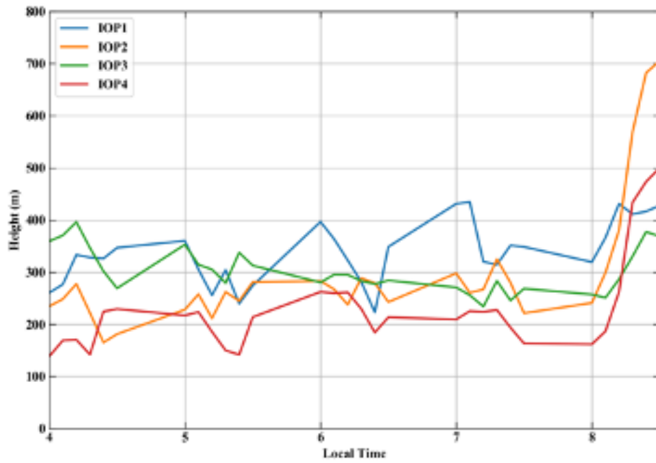
Figure S3 Transition from night to day PBL of the ceilometer for 4 IOPs, averaging every 10 minutes.
