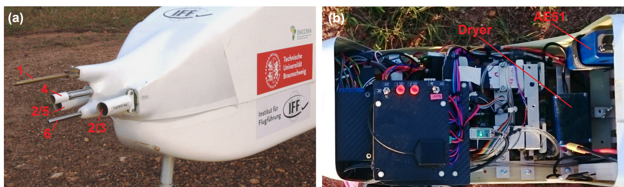
Figure 2. (a) The nose of the aircraft is equipped with meteorological sensors for calculating the three dimensional wind vector with one multihole probe (number 1), the temperature (number 2–4) and the humidity (number 4 and 5). The air probe is sampled with one aerosol inlet (number 6) mounted at the tip of the aircraft's nose. (b) The micro aethalometer AE51 is installed in the front compartment of the aircraft for adjusting the centre of gravity. The air stream is dried with silica gel before measuring (see the blue box close to the AE51).
