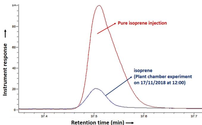
Figure S5: Sample chromatogram of the isoprene peak resolved on the Alumina PLOT column at a retention time of 37.5 min in the air collected from the plant chamber experiment overlaid with the peak from pure isoprene vapours injected to determine the retention time of isoprene.
