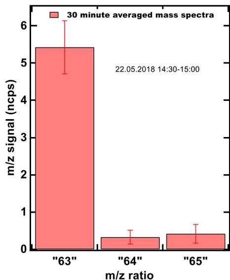
**Figure S4 (b): 30 min averaged PTR-MS mass scan of the output air from the branch cuvette system during the afternoon period on 22.05.2018 of m/z 63, 64 and 65; error bars reflect combined instrumental precision error and emission variability.**
