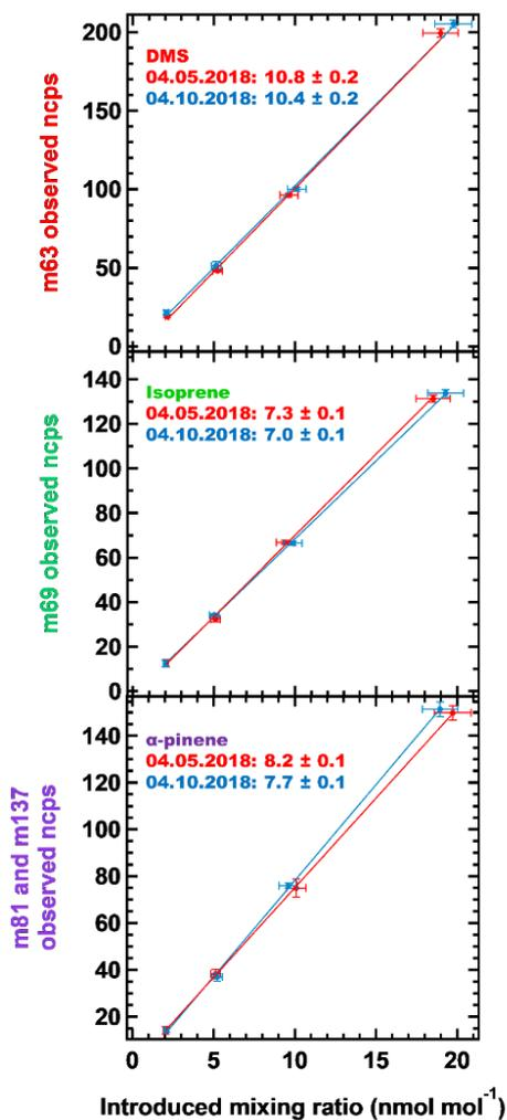
Figure S2: Results of calibration experiments performed on 4 May 2018 and 4 October 2018 for DMS, isoprene and  $\alpha$ -pinene illustrating the excellent linearity and low drift in sensitivity of the PTR-MS for these compounds
