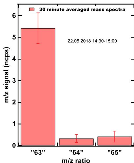
**Figure 1.** 30 min averaged PTR-MS mass scan of the output air from the branch cuvette system during the afternoon period on 22.05.2018 of  $m/z$  63, 64 and 65
