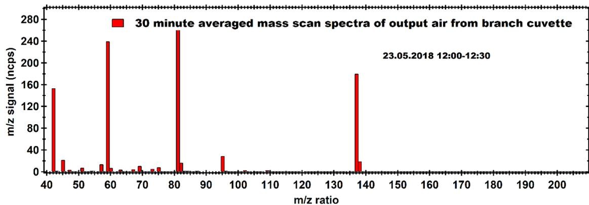
5 Figure S3: A typical 30 min averaged PTR-MS mass scan of the output air from the branch cuvette system during the afternoon period after subtraction of input background air signals showing the ion signals observed in the mass range  $m/z$  40 to  $m/z$  210.
