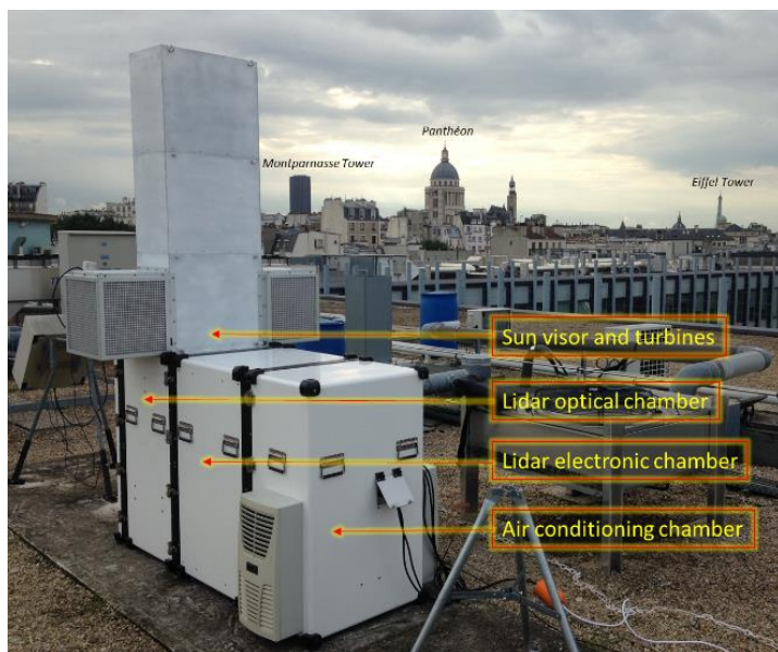
Figure 1: LAASURS system on the Paris Sorbonne University rooftop
