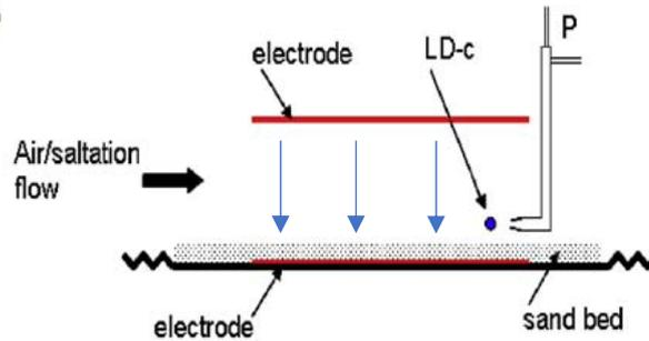
**Figure R3.** (adapted from Rasmussen et al., 2009) Two parallel-plate electrodes are used to generate the external electric field.
