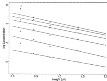
**Figure R6. (adapted from Sørensen and McEwan, 1996).** Concentration profiles (grains/cm<sup>3</sup>) calculated by the McEwan-Willetts model (squares) and the fitted curves of the type given by Eq. (5) (full drawn lines). The grain concentration increases with shear velocity ( $U^*=28, 35, 49, 66, 79, 90$  cm/s).
