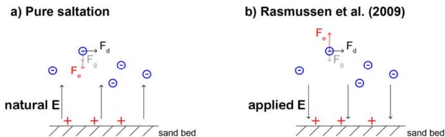
**Figure R1.** Schematic of the forces acting on the negatively charged (on average) saltating particles. Here,  $F_d$ ,  $F_g$ , and  $F_e$  denote the drag force, gravitational force, and electrostatic force. (a) The downward-pointing  $F_e$  exerted by the natural electric field produced by the charged sand particles. (b) The upward-pointing  $F_e$  exerted by the man-made electric field.
