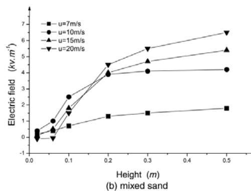
**Figure R4.** (adapted from Zheng et al., 2003) Measurement of magnitude of electric field strength versus height in wind-blown sand cloud with mixed sand in a wind tunnel.
