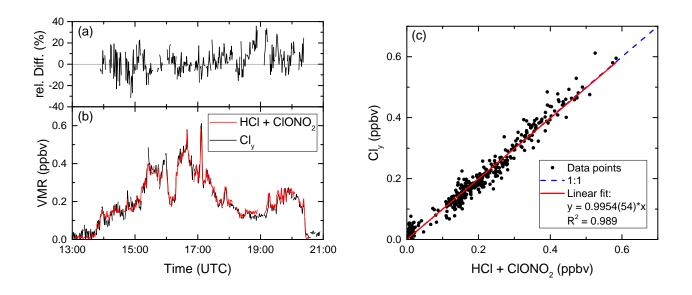
**Figure 2.** Comparison of the sum of HCl and ClONO<sub>2</sub>, measured by AIMS, to  $Cl_y$ , inferred from GhOST measurements, during Flight 04 on 17 December 2015. (a) Difference between both curves relative to  $Cl_y$  and (b) timeline of mixing ratios over the whole course of the flight. (c) Correlation between added AIMS measurements and  $Cl_y$ .
