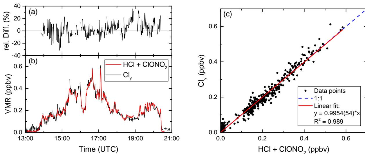
**Figure 2.** Comparison of the sum of HCl and ClONO<sub>2</sub>, measured by AIMS, to Cl<sub>y</sub>, inferred from GhOST measurements, during Flight 04 on 17 December 2015. (a) Difference between both curves relative to Cl<sub>y</sub> and (b) timeline of mixing ratios over the whole course of the flight. (c) Correlation between added AIMS measurements and Cl<sub>y</sub>.
