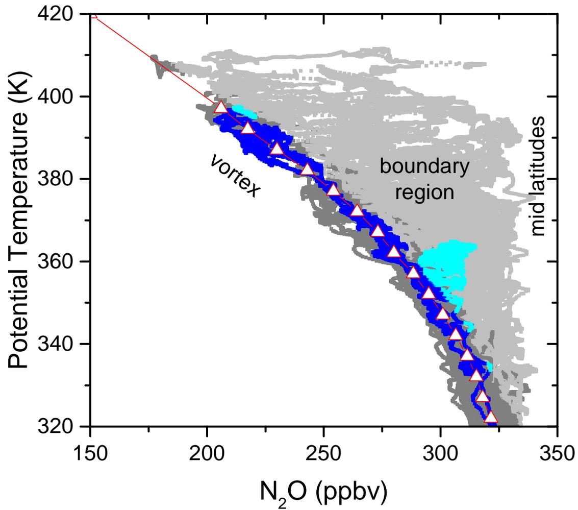
**Figure 3.** Profiles of  $N_2O$  versus potential temperature for the whole PGS campaign (grey) and for the selected Flight 14, of 26 February 2016 (blue), above 320 K. The derived vortex reference profile is illustrated by the triangles, connected by straight red lines. Dark and light subsets of the grey and blue points indicate the assigned vortex air and extra-vortex air property, respectively.
