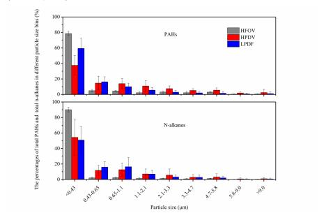
Figure 6 The distribution of total PAHs and total n-alkanes in different particle size bins (%)
