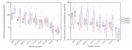
Figure 7 Emission ratiosof total PAHs (in µg (g<sup>-1</sup> PM)) and n-alkanes (in mg (g<sup>-1</sup> PM)) in size-resolved particles
