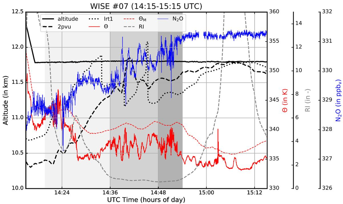
**Figure 4.** Time series of measured  $N_2O$  (blue) and potential temperature  $\Theta_M$  (red solid) as well as modeled potential temperature  $\Theta$  (red dashed), Richardson number  $RI$  (gray dashed), and altitude of the dynamic tropopause (2 pvu, black dashed) and the first lapse rate (lrt1, black dotted) tropopause between 14:15 and 15:15 UTC during WISE RF07. Black solid line shows the altitude of the aircraft, the gray areas indicate the time periods discussed in the text.
