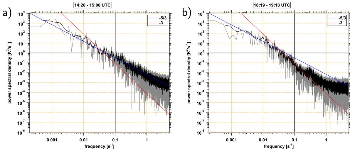
**Figure 6.** Power spectral densities of measured potential temperature from HALO for selected time periods: a) 14:20 - 15:00 UTC and b) 18:19 - 19:18 UTC. Black solid lines are introduced for better comparability, red solid lines shows a line with a slope of  $k = -3$ , blue solid line shows a line with a slope of  $k = -5/3$ .
