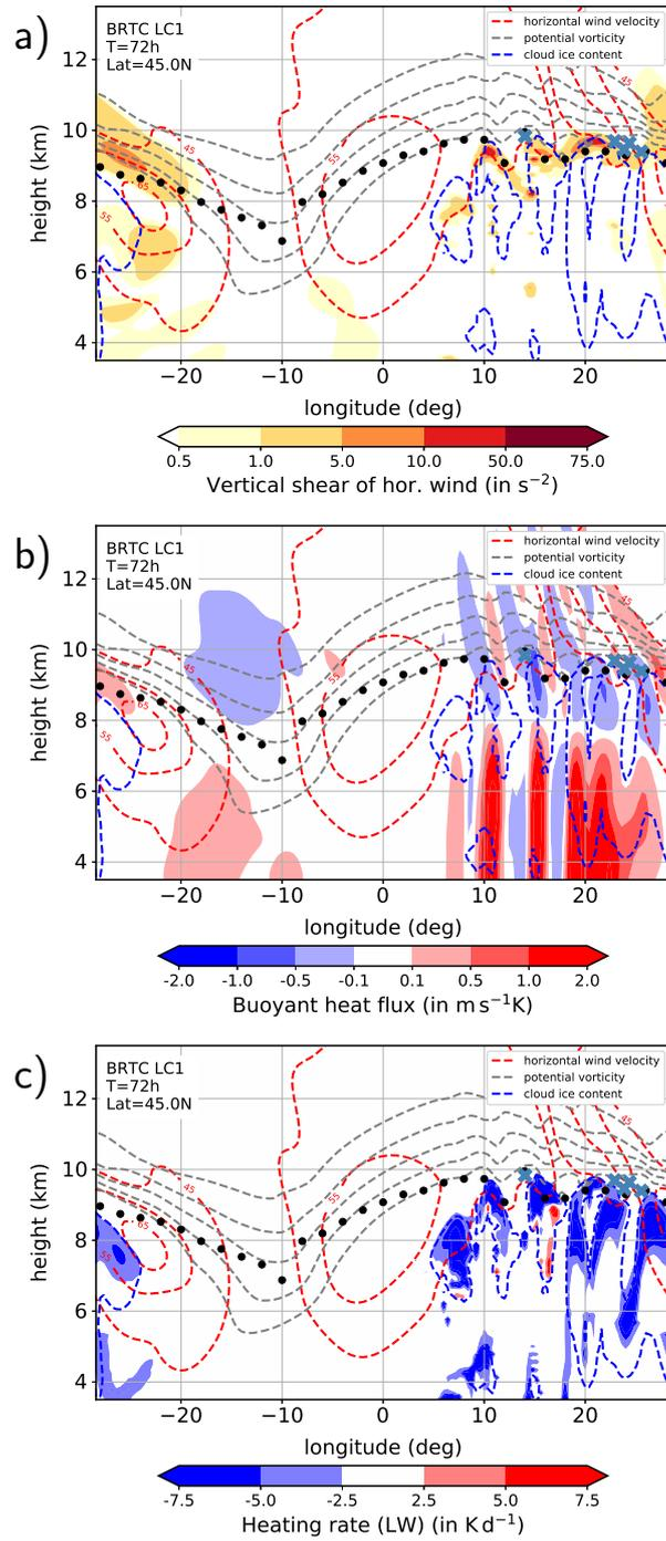
**Figure 14.** Zonal cross sections of a) vertical shear of horizontal wind  $S^2$ , b) buoyant heat flux  $w'\Theta'_v$ , and c) long wave heating rate  $D\Theta_{LW}/Dt$  at  $45^\circ N$  and after 72 h of model integration. For the description of isolines it is referred to Figure 11.
