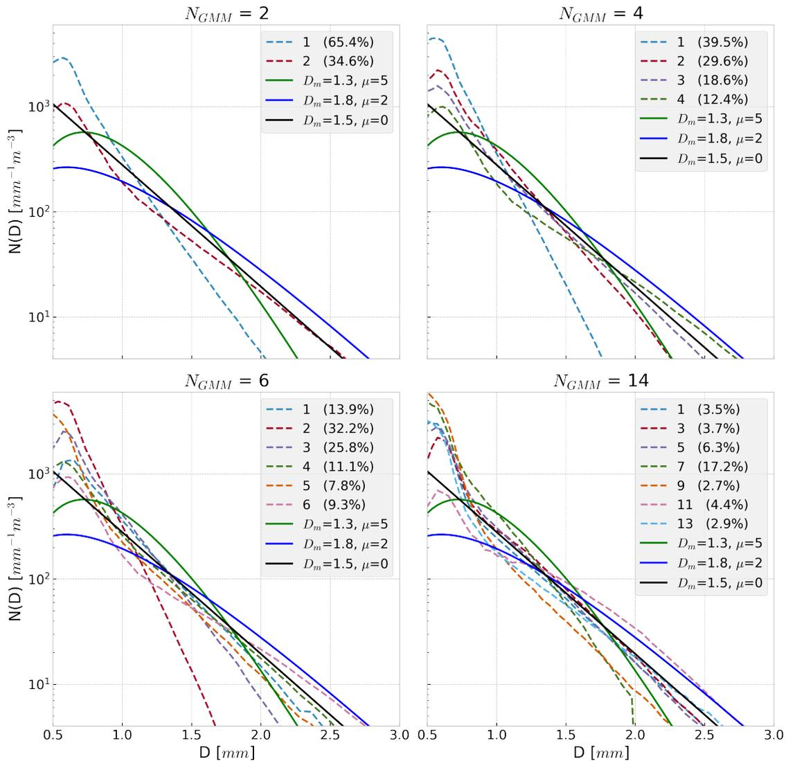
**Figure 7.** Panels show resultant DSDs for different GMM realizations (dashed lines) ranging from  $N_{GMM}$  of 2 to 14. The last panel shows only odd numbered GMM states to reduce clutter. Each panel has an identical set of NG curves with different  $\mu$  and  $D_m$  values (solid lines) for the sake of comparison. All curves have equal RWC. The frequency of occurrence for each GMM shape is given in the legend.
