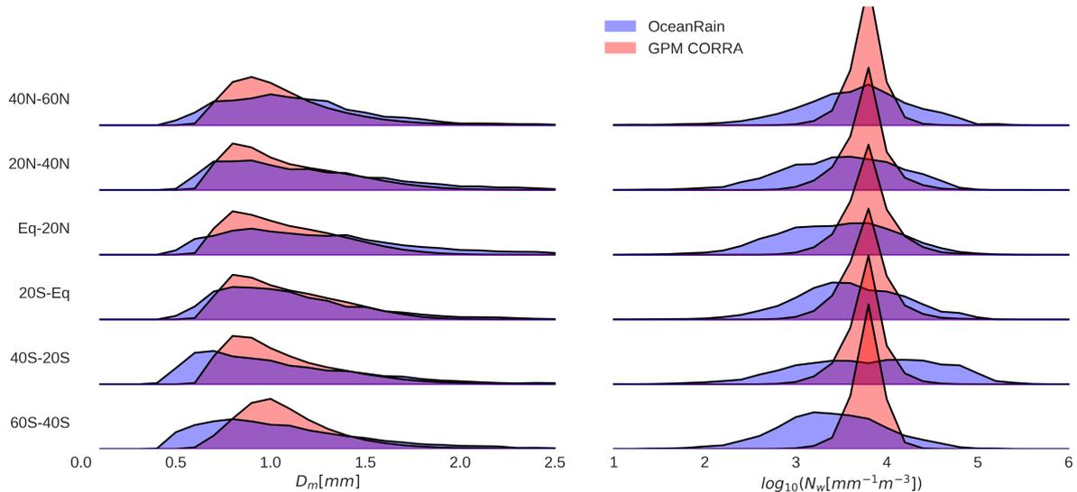
**Figure 5.** Normalized histograms of  $D_m$  (left) and  $\log_{10}(N_w)$  (right) for GPM CORRA and OceanRAIN, separated by latitude. All histograms use a linear y-axis of height 20%. GPM data are from the 3B CMB monthly gridded product.
