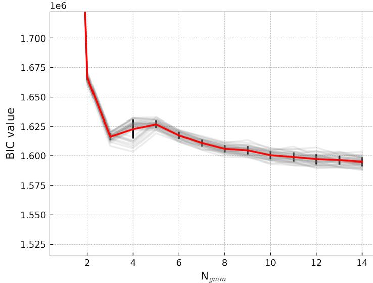
**Figure 8.** Bayesian Information Criterion (BIC) for different  $N_{GMM}$  choices applied to OceanRAIN. The mean BIC is shown in red with the standard deviation in black. Gray lines indicate GMM tests with limited samples, each a randomly chosen subset making up a third of the total data set.
