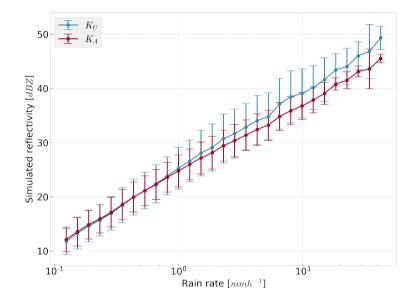
Figure 10. Simulated radar reflectivities at the two DPR frequencies,  $K_U$  and  $K_A$  bands, shown as means (dots) and standard deviations ( $\pm 1\sigma_A$  shown as bars) binned by rain rate. The rain rate and the DSD are directly from OceanRAIN observations.
