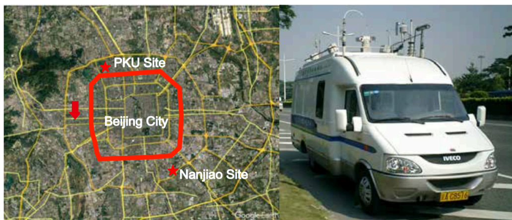
Figure 1. The measurement route (left) and the mobile measurement platform (right). The route started from the Peking University (PKU), driving counter-clockwise around (indicates by the red arrow) the 4th Ring Road of Beijing (circumference ~65 km) before returning to PKU. The red line represents the 4th Ring Road of Beijing, and the red stars show the ground-based observation sites (PKU and Nanjiao).
