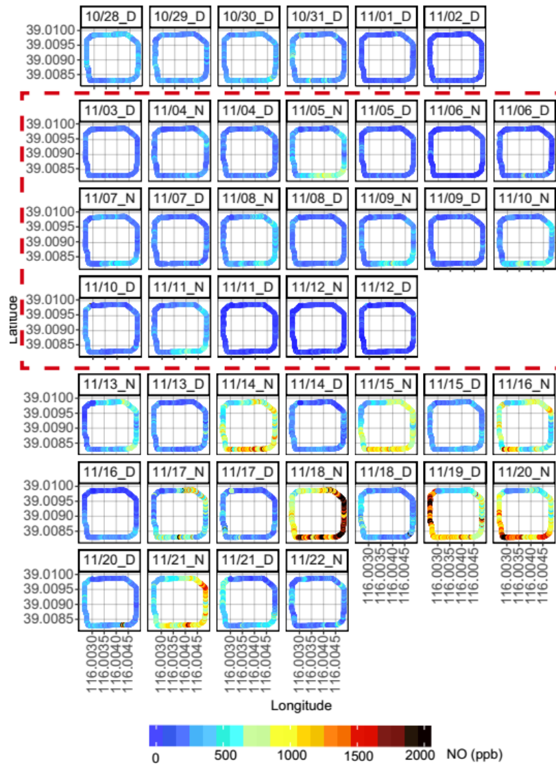
Figure 4. The spatial distributions of NO around the 4th Ring Road of Beijing from 28 October to 22 November 2014. The subtitle for each circuit indicates the observation time in the form “MM/DD_Day, Night”. The red dotted rectangle area indicates the full-APEC period.
