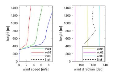
Figure 3: Mean wind speed (left panel) and wind direction (right panel) profiles in the considered scenarios and sensitivity experiments.
