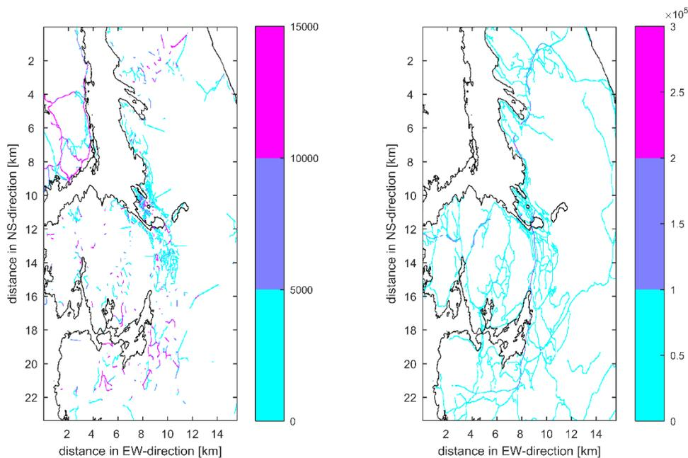
5 **Figure A1:** Annual mean daily traffic flow in vehicle meters ( $N_i \cdot l_i$ ) in each PALM grid cell for side-streets (left panel) and main roads (right panel). Both colour shadings have the unit [m]. Roads in the left panel that are appearing to go straight into mountainous areas are sporadically used small utility roads. For simplicity of the underlying traffic model they are indicated as straight roads instead of following their actual path. Emissions from these roads are negligible.
