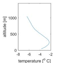
temperature  $[^{0} C]$ Figure 2: The mean vertical temperature profile used for nudging in the PALM domain.
