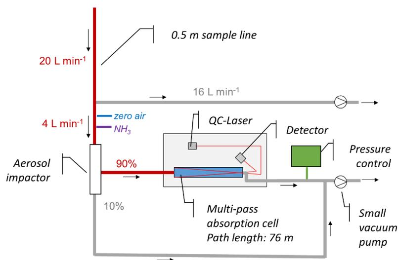
10 **Figure 2: Setup of the QC-TILDAS on the Twin Otter aircraft for  $\text{NH}_3$  measurements at 1 Hz sample frequency. The commercially available QC-TILDAS was modified using a smaller vacuum pump, a pressure controller and a custom made PFA aerosol impactor. A bypass system was used to generate a higher flow rate through the inlet line. See text for a detailed description of the setup.**
