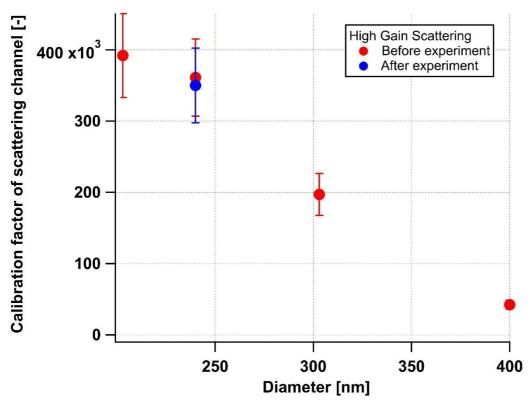
Figure S2 PSL calibration for high gain scattering channel before and after the investigation.
