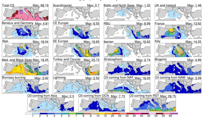
**Figure 5.** Average MDA8 O<sub>3</sub> mixing ratio (upper left panel) and contribution of each tagged O<sub>3</sub> region and source over the Mediterranean Sea for the April-September 2010 period. The unit is ppb
