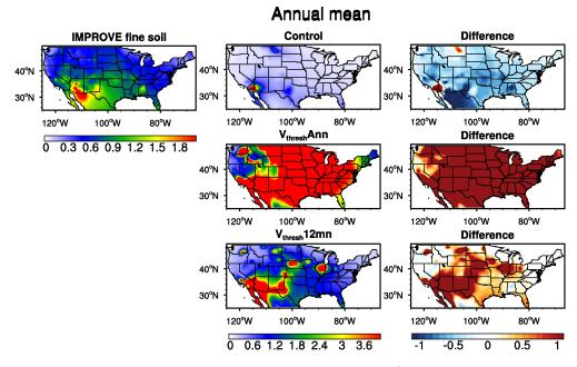
1420 Figure 9. Annual mean surface fine dust concentration ( $\mu$ g m<sup>-3</sup>) from IMPROVE stations 1421 (left column) and three simulations (middle column) and the differences between model 1422 and observation (right column) for 2002-2015.
