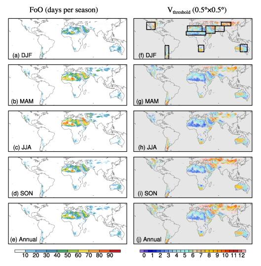
1318Figure 1. (a)-(e) Frequencies of occurrence (FoO; unit: days per season) in each season1319and annual mean. (f)-(j) Threshold of wind erosion ( $V_{threshold}$ ; unit: m s<sup>-1</sup>) derived from1320satellite products and reanalyses for each season and annual mean. Black boxes in (f)1321denote nine dusty regions as listed in Table 1.
