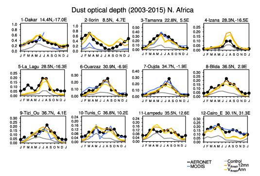
1469Figure 11. Seasonal cycle of DOD over 12 AERONET SDA sites (see Fig. S5 in the1470Supplement for locations) from the Control (grey),  $V_{thresh}12mn$  (orange), and  $V_{thresh}Ann$ 1471(yellow) simulations, along with DOD from MODIS (blue), and COD from AERONET1472(black dotted line). All values are averaged over 2003-2015. The location (lat/long) and1473the name (due to space, only first seven characters are shown) of the sites are listed at the1474top of each plot.
