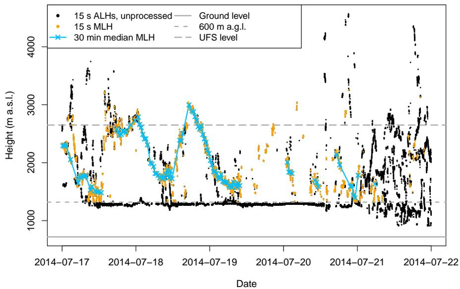
**Figure 2.** Post-processing of the ceilometer-based aerosol layer heights (ALHs), which were used to determine the mixing layer height (MLH) at GAP, illustrated for the period from 17 to 21 July 2014. From the MLH, outliers have been removed. Points of the 30 min median MLH were connected by a line if separated by maximum 3 h.
