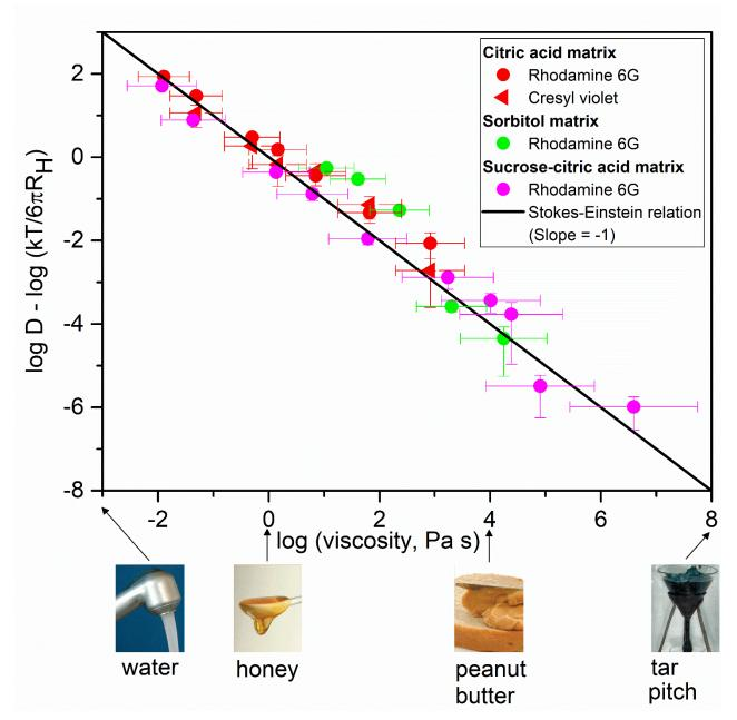
Figure 2. Plot of log (D) – log (kT/ $6\pi$ R<sub>H</sub>) as a function of log ( $\eta$ ) for measurements shown in Fig. 1. Viscosities ( $\eta$ ) were determined from relationships between viscosity and aw (Figs. S7 -S9). T corresponds to the experimental temperature and R<sub>H</sub> corresponds to the radius of each diffusing species (see Table S5). The x-error bars were calculated using the uncertainty in aw at which the samples
