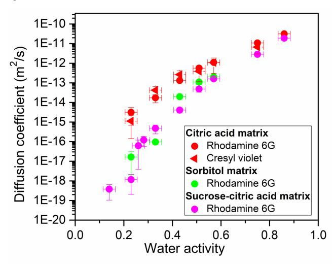
Figure 1. Measured diffusion coefficients of fluorescent organic molecules in various organic matrices as a function of water activity (aw). X-error bars represent the uncertainty in the measured aw (0.025) and y-error bars correspond to two times the standard deviation in the diffusion measurements. Each data point is the average of a minimum of four measurements. Indicated in the legend are the fluorescent organic molecules studied and the corresponding matrices.
