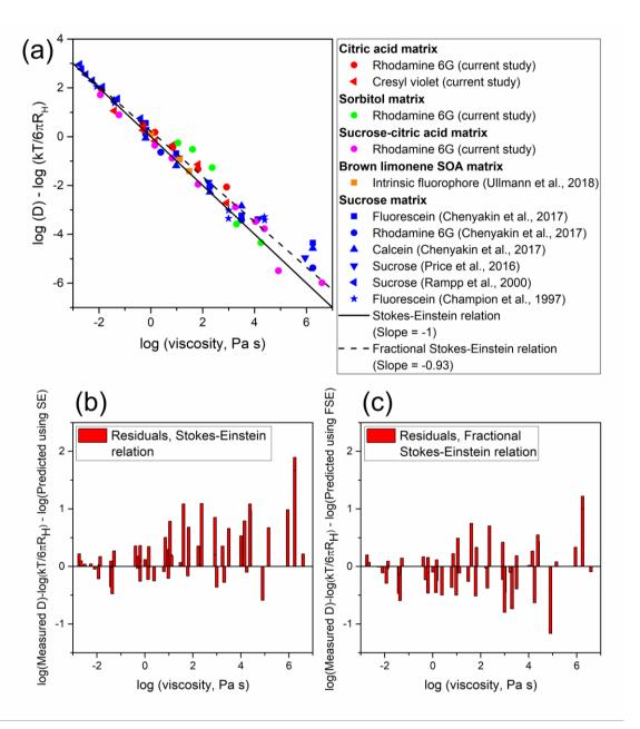
Figure 3. a) Plot of log (D) – log (kT/6 $\pi$ R<sub>H</sub>) as a function of log ( $\eta$ ) for new measurements reported in this work and literature data. Indicated in the legend are the diffusing organic molecules studied and the corresponding matrices. T corresponds to the experimental temperature of each diffusion measurement and R<sub>H</sub> corresponds to the radius of each diffusing species (Section S2 and
