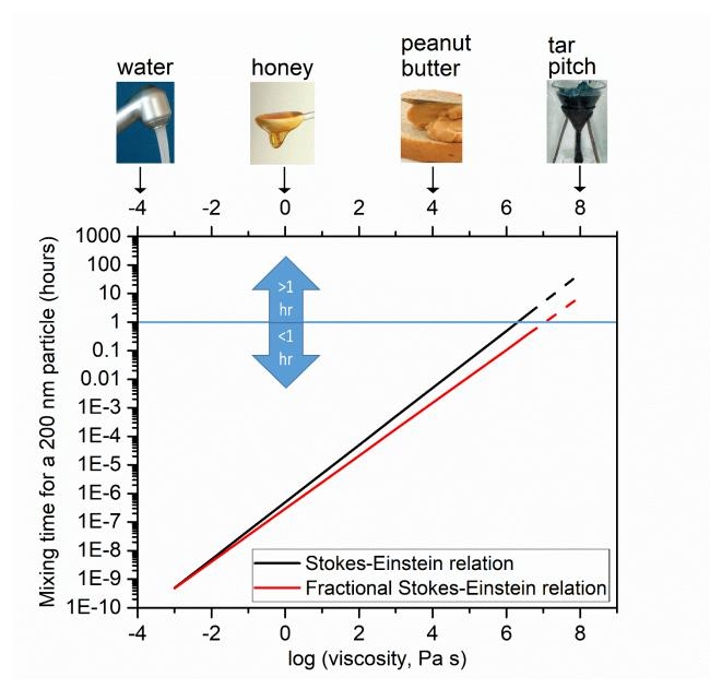
Figure 4. Mixing times of organic molecules within a 200 nm particle as a function of viscosity using the Stokes-Einstein relation (black line) and a fractional Stokes-Einstein relation (red line). The dashed lines indicate that the relations were extrapolated to viscosities beyond the tested range of viscosities ( $\geq 4 \times 10^6$  Pa s).
