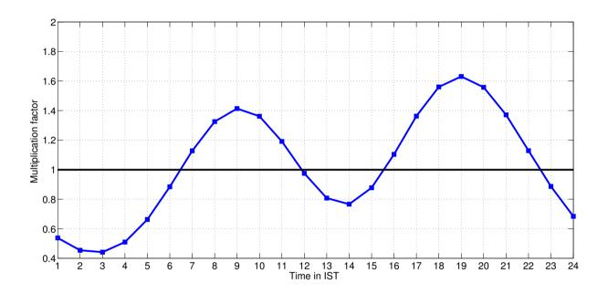
Figure 1. The prescribed diurnal variation to the emissions of BC,OC, Sulfate, SO<sub>2</sub>, CO, NO and NO<sub>2</sub> in this study.
