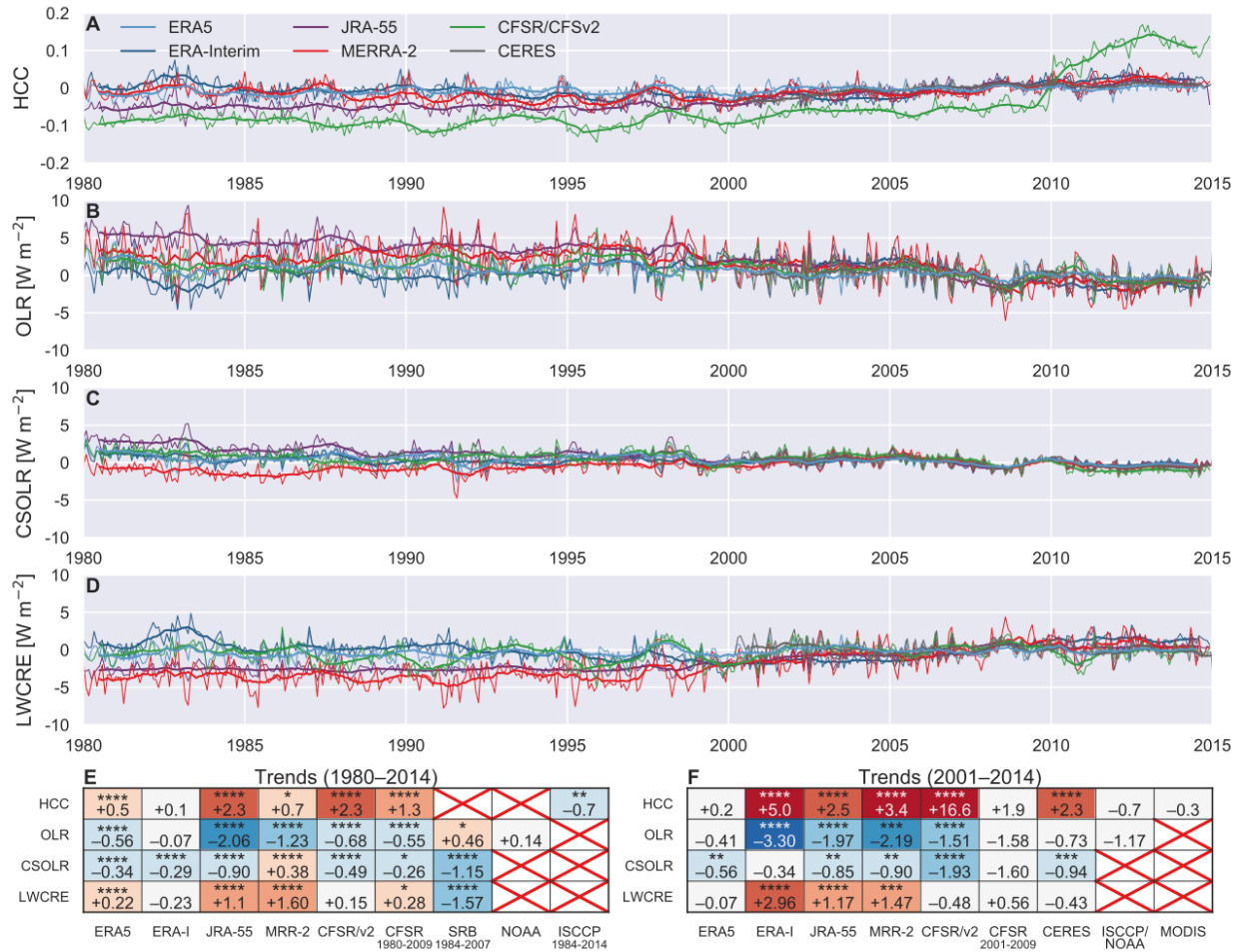
Figure R5: Time series of deseasonalized anomalies in (A) monthly mean high cloud cover (HCC), (B) monthly mean OLR, and (C) monthly mean LWCRE averaged over the inner tropics (10°S–10°N) for 1980–2014 based on ERA5 (cyan), ERA-Interim (blue), JRA-55 (purple), MERRA-2 (red), and CFSR/CFSv2 (green). Observational analyses from CERES SYN1Deg (A; March 2000–December 2014) and CERES EBAF (B and C; March 2000–December 2014) are shown for context. Anomalies are calculated relative to the mean annual cycle during 2001–2014. Thick lines show time series after applying a 12-month uniformly-weighted rolling mean. Trends are listed for annual-mean anomalies during the (D) 1980–2014 and (E) 2001–2014 periods in percentage points per decade for HCC and units of W m^{-2} per decade for OLR, clear-sky OLR, and LWCRE. Stars indicate statistical significance at the 90% (*), 95% (**), 99% (***), and 99.5% (****) confidence levels. Light grey shading indicates that the 90% confidence interval of the Theil–Sen slope contains zero. Blue colors mark negative trends and red colors positive trends, with darker shades indicating larger trend magnitudes (0 to 1, 1 to 2, 2 to 3, and greater than 3).
